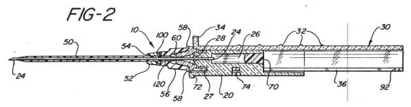
Figure 2 depicts a cross-sectional view of Van Heugten's catheter assembly 10. *Id.* at 2:9–10, 19–21. In particular, Figure 2 illustrates catheter assembly 10 with catheter 50 and needle 24, which needle guard 30 covers upon retraction of needle 24 to prevent inadvertent needle injury to the user or others. *See id.* at 2:36–39, 3:34–58. Catheter assembly 10 also includes valve membrane 110, which is illustrated in Figures 4a and 4b, which we also reproduce, below:
