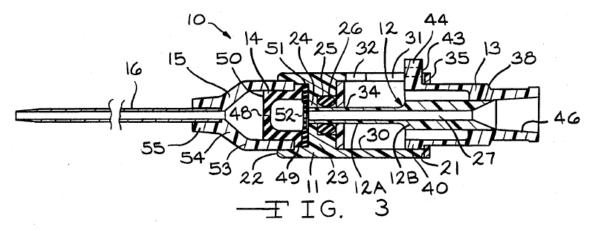
Figure 3 of Rogers illustrates check valve assembly 10 including slit 48 in valve 14, and sliding separator 12, in comparison with Figure 2 from Tauschinski below.
