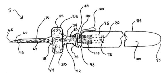
The sole Figure from Lynn, above, depicts vascular access system 5 including a needle protective device (needle receptacle 84) for receiving spring biased needle 60. According to Lynn, when a user depresses button 120, spring 105 is released from a compressed state retracting needle 60 into receptacle chamber 100. *Id.* at 7:15–26.
