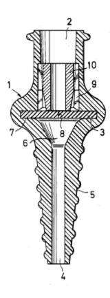
Tauschinski's valve, shown above in Figure 2, includes valve disc 3, slit 8, and slidable actuator 10.
