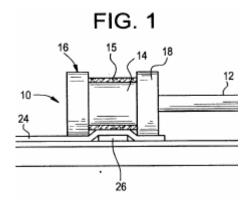
Portions of the rubber cushion [15] directly over the fastening means [26] are compressed, while portions of the rubber cushion [24] adjacent to the fastening means conform to the underlying second thermoplastic sheet [22] and in sufficiently tight contact therewith to expel air from between the overlapping portions of the thermoplastic sheets so as not to allow formation of air pockets or bubbles.
