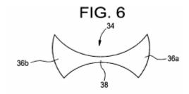
opening 34 comprises large openings 36a and 36b and a restricted opening portion 38 between 36a and 36b. It was found that the restricted opening portion 38 still allows sufficient outflow of heated air to sufficiently soften the overlapping portion of the thermoplastic sheets over and under the fastening means in order to weld the thermoplastic sheets together over the interposed fastening means.
