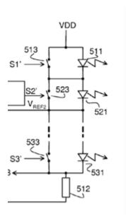
Typical problems appearing in the documents with this symbol are: accommodation of potential in a chain of series-connected LEDs, adaptation of the number of LEDs to various supplied voltages.
