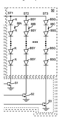
RGBs, current mirroring, active current balancers, minimum voltage selectors, in general when the parallel branches are gated for some purpose.
