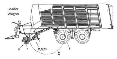
Pick up 6 with feeler wheel 7 and cutting device 11 comprising the conveying rotor 12 and the knife assembly 13 in the cutting frame.
