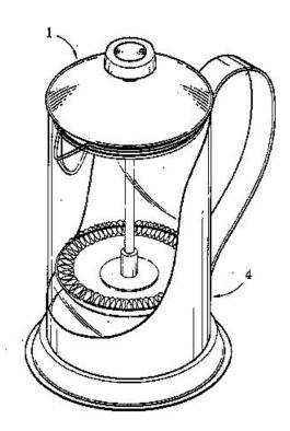
Example of a coffee machine of the type "French press" (from US6186052 by Huang)
