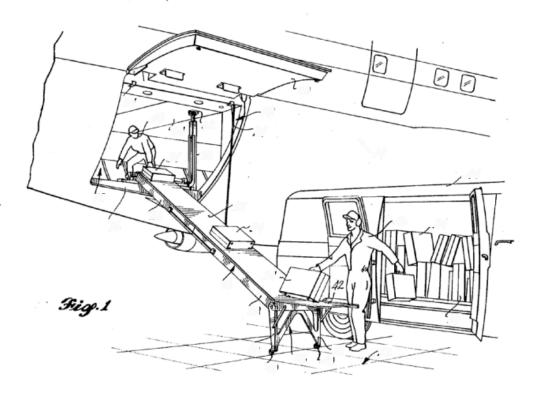
{Supply vehicles specially adapted for transporting catering to and loading into the aircraft}
