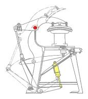
{Fluid-control mechanisms for controlling the ironing pressure or the movement of the pressure member}
