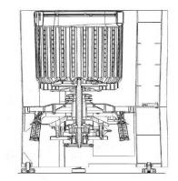
{Damping vibrations by displacing, supplying or ejecting a material, e.g. liquid, into or from counterbalancing pockets}
