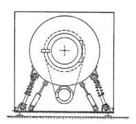
{Damping vibrations by displacing, supplying or ejecting a material, e.g. liquid, into or from counterbalancing pockets}
