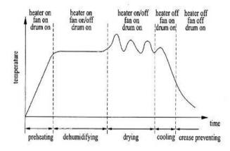
The above diagram represents a typical drying method for laundry dryers, belonging to <u>D06F 58/30</u> in which, during the drying process, the heater and the blower fan are subsequently turned ON/ OFF while the drum is rotated. It is noted that <u>D06F 58/30</u> relates to methods for treating the laundry
