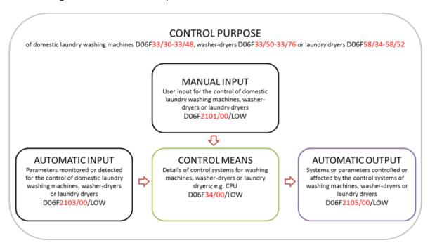
A controlling process for a laundry treating apparatus (e.g. a washing machine) has a specific "control purpose" and implies the presence of a "control means" (e.g. a CPU), whereby the control means is usually a control unit which comprises a user interface (e.g. a control panel) and several sensors for the automatic detection of e.g. temperature, pressure, liquid level, etc.
