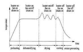
The above diagram represents a typical drying method for laundry dryers, in which several laundry treating steps are performed, for example during the drying process the heater and the blower fan are subsequently turned ON/OFF while the drum is rotated.
