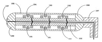
Vibrating metal strip in flow path: US4420983 (fig.11):
