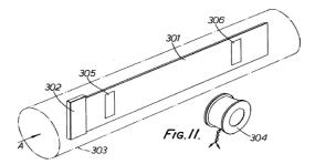
Vibrating cylinder in flow path: US4420983 (fig 1):
