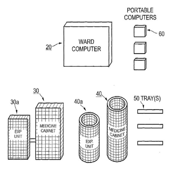
Example 2: Drug dispensing control system has a drug-dispensing unit with canister receiving a prescribed amount of medication from a prescription filling system. The canister includes a single dose
