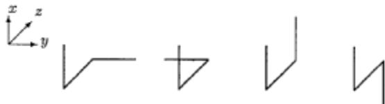
Fig. 1. Basic wire structures. Two chiral cranks of opposite handedness (enantiomorphs), a non-chiral staple, and a non-chiral crank.
