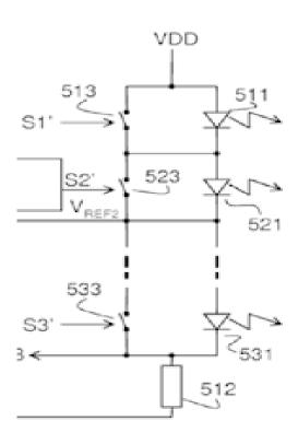
Typical problems appearing in the documents with this symbol are: accommodation of potential in a chain of series-connected LEDs, adaptation of the number of LEDs to various supplied voltages.
